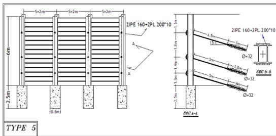
Fig. 12: An example of soldier pile valuation type plan (depth of 6 meter, type 5)
