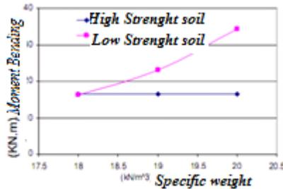
Fig. 7: Chart of bulk density impact on the amount of moments
