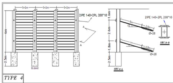
Fig. 11: An example of soldier pile valuation type plan (depth of 6 meters type 4)
