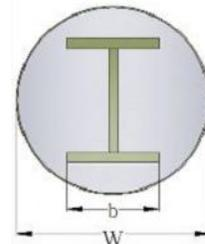
Fig. 1: Effective width and proximity coefficient
