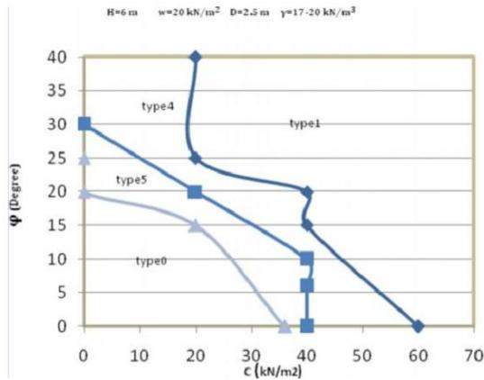
Fig. 10: A sample of soldier pile valuation type graph (depth of 6 meter for live load 20 KN/M<sup>2</sup>)
