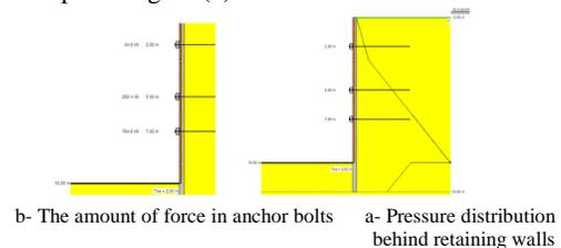
Fig. 4: An example of software output a- pressure distribution behind retaining walls b- the amount of force in anchor-bolts
