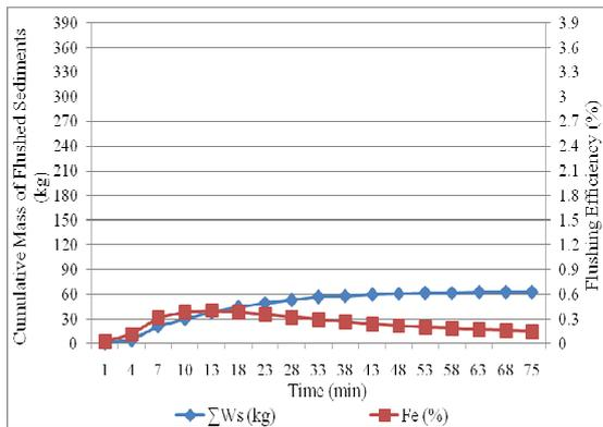
Figure 8c: Variation of Fe and  $\Sigma W$  against time for Run no. 3
