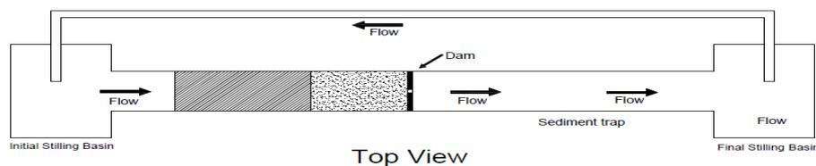
Figure 1b: Top view of Experimental model
