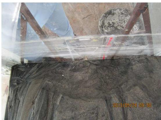
Figure 6: Flushing cone formed during Run no. 3 (view from top)
