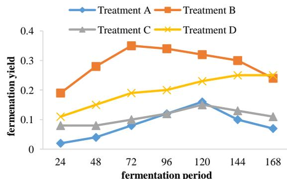
Figure 6: Ethanol yield ( $Y_{p/s}$ ) produced from the various Treatments
