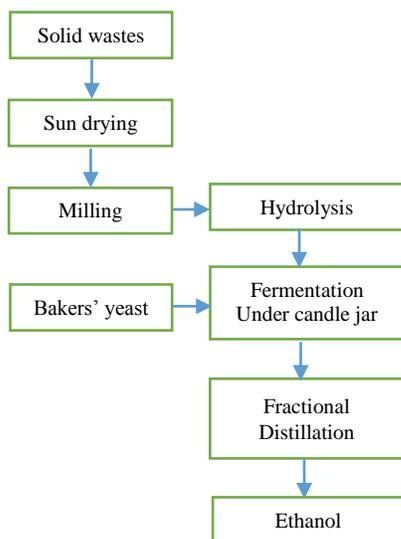
Figure 2: Flow chart of ethanol production
