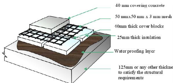
Figure 4: Detailed arrangement of the insulation system proposed over reinforced concrete slabs
