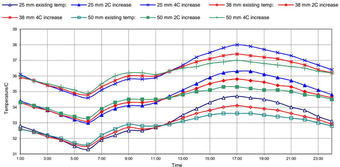
Figure 8: Upper floor slab soffit temperature variation with global warming
