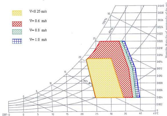
Figure 3: Modified comfort zone when the out door temperature increase by 4°C
