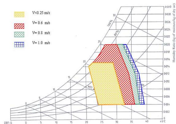
Figure 2: Modified comfort zone when the outdoor temperature increase by  $2^{\circ}\text{C}$
