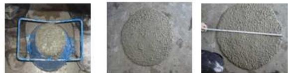
Figure 3: How to carry out the slump flow test
