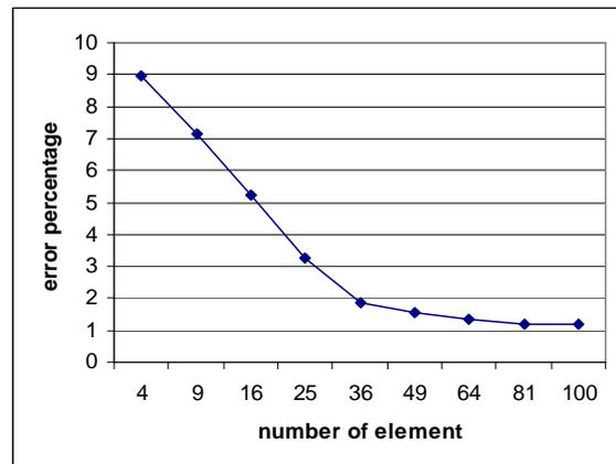
Figure 8: Error changes for different plate elements
