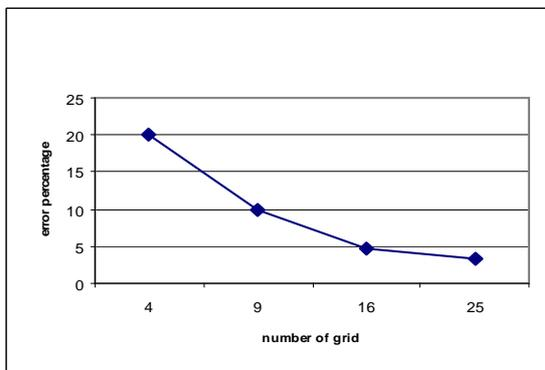
Figure 6: Error changes for increasing of plate grids
