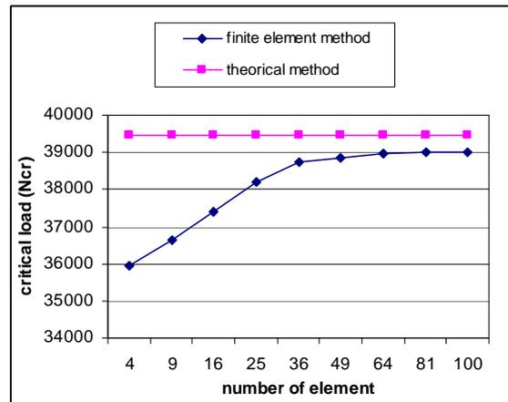
Figure 7: Critical load of plate for different number of elements
