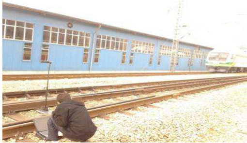
Figure 8. Noise Recording by railway vehicle passing in the tangent track
