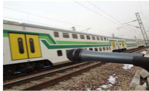
Figure 9. Noise Recording by railway vehicle passing in the curve
