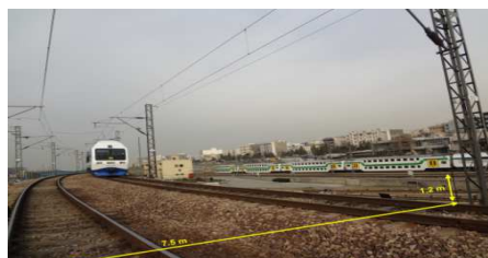
Figure 6. Microphone position in accordance with the standard ISO 3095 in the curve
