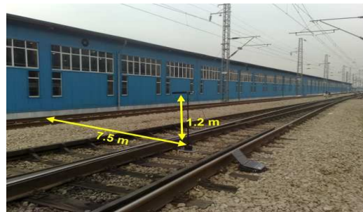
Figure 5. Microphone position in accordance with the standard ISO 3095 in the tangent track
