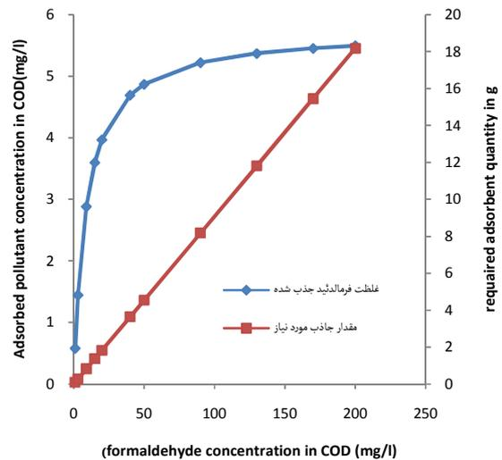
Fig.6: Prediction of removable formaldehyde and the required adsorbent rate in various formaldehyde concentrations
