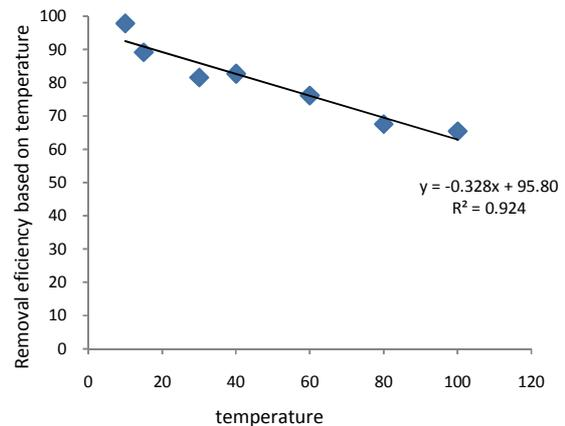
Fig.2: Formaldehyde removal efficiency by activated carbon on different temperatures
