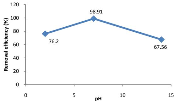
Fig.1: Formaldehyde removal efficiency changes in adsorption by activated carbon in different pHs
