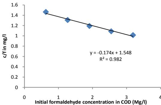
Fig.5: Resulting plotted regression of  $\frac{1}{k \times f_{max}}$  against  $\frac{1}{f_{max}}$
