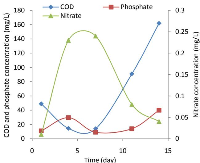
Fig 4. The reduction rate of COD, phosphate and nitrate based on different time intervals
