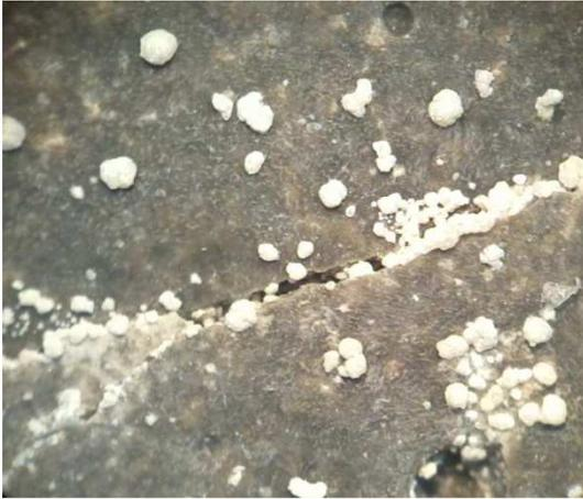
Figure 2: Microbial persipitation of calcium carbonate around of a concrete crack
