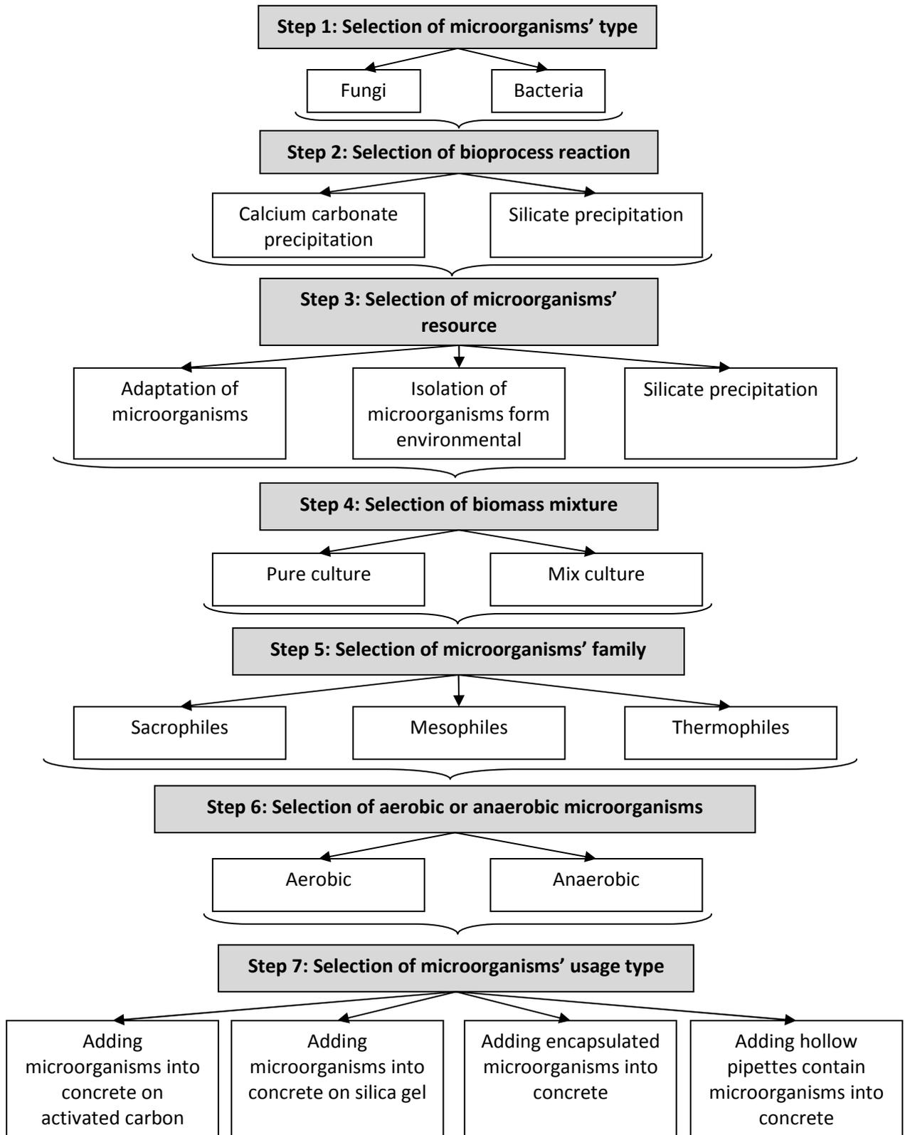
Figure 1: Different steps to conduct a study on biological self-healing concrete
