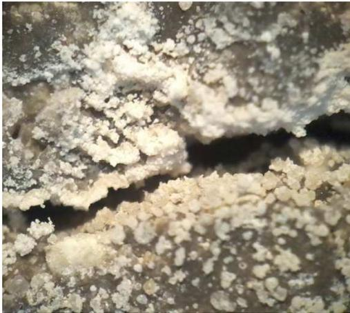
Figure 4: Microbial persipitation of calcium carbonate around of a concrete crack
