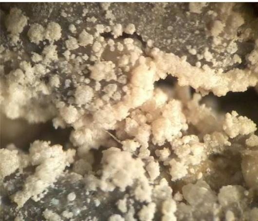
Figure 3: Microbial persipitation of calcium carbonate around of a concrete crack
